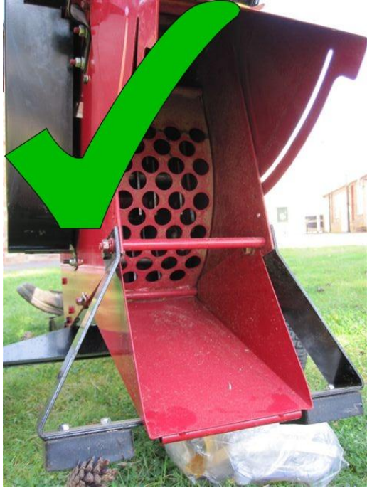
Correct Fitting position of Bottom Discharge Chute
