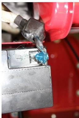
19. Screw live and neutral cables into place on battery (marked black and red on the battery).
