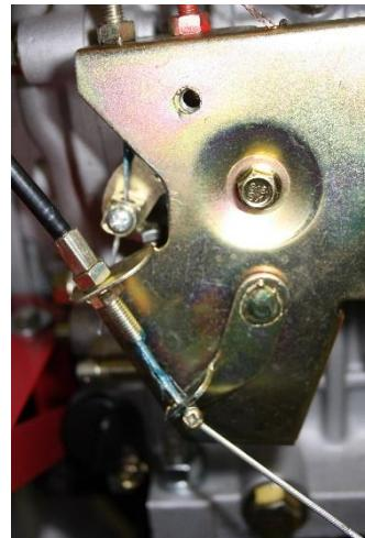
Deadman's Handle Cable – Loosen bottom nut and tighten top nut half turn.
