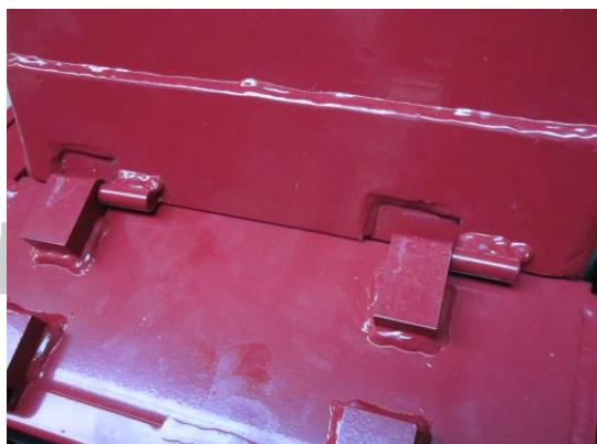
10. Install discharge chute following the same procedure as the Feed hopper ensuring the two retaining bolts are fitted and fully tightened once it is in position.
