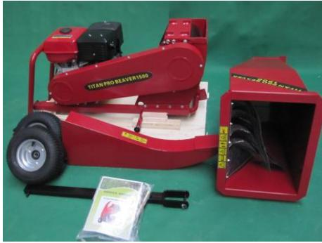
4. To enable the removal of the main body of the chipper carefully prise off the shipping blocks as shown below, once this has been done invert the machine on end as shown in the photo below.
