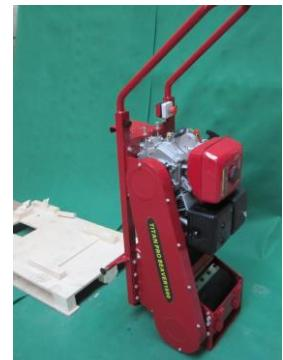
5. Bolt on both wheels and position the machine in a horizontal position
