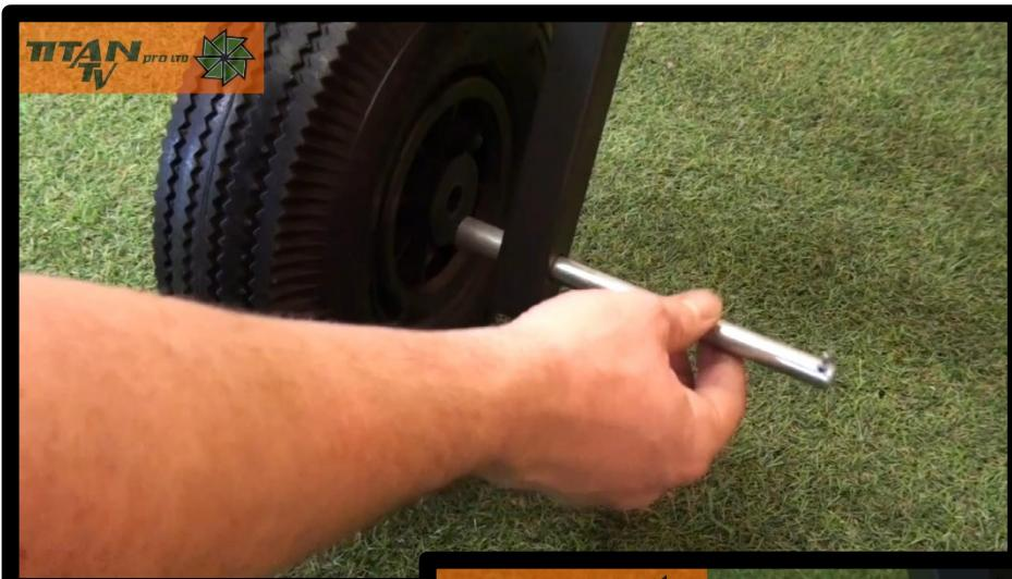
You can then rest the frame on the wheel and ready the other **1 x wheel spindle spacer**.
