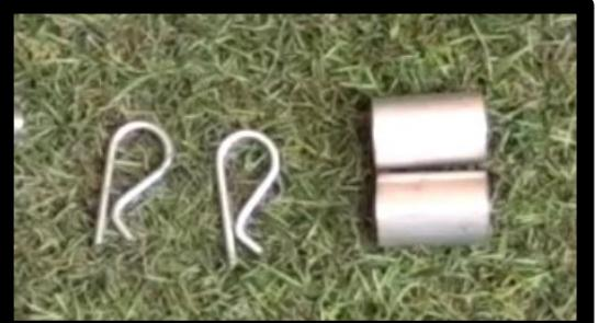
Start with **1 x Wheel**, **2 x "R" Clips**, **2 x wheel spindle spacers** and **1 x wheel spindle**.
