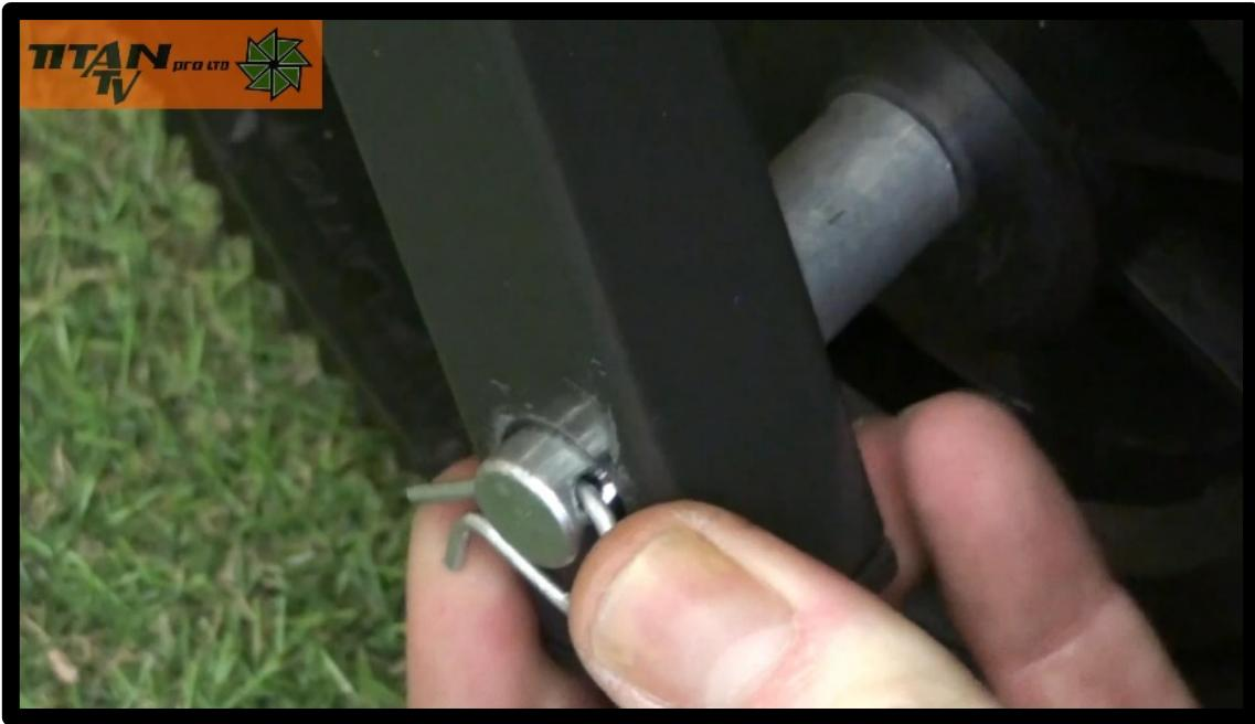
To secure the wheel and spindle assembly, find the final **1 x “R” clip** and push this through the exposed hole on the outside of the spindle.
