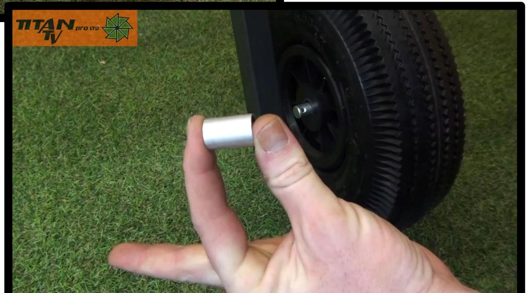
Once the spacer lines up then push the spindle through the wheel, spindle and leg, so that the spindle protrudes enough on the outside – *You should be able to see the small hole on the spindle when the “R” clip will be inserted. (See picture on the next page for reference).*
