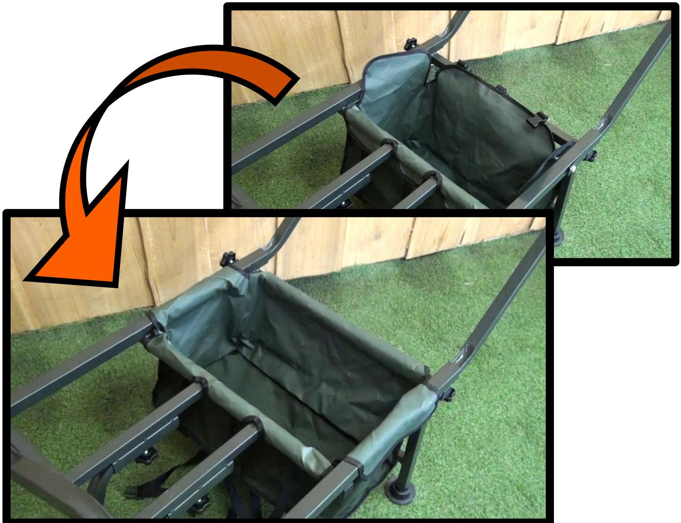
Loop the securing straps underneath the frame and leading to the rear of the trolley. Lay them out straight and untangled, as the picture below.
