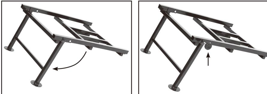
2. Insert the two L shaped sections into the main frame, and tighten using two plastic knobs as shown below.
