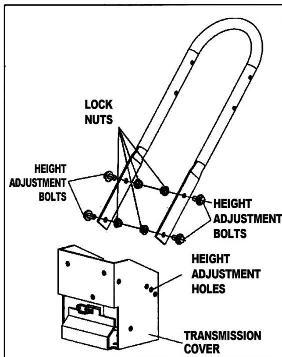
**STEP 3: Attach handle bar to the Tiller**
