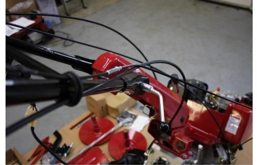
8. Remove adjustment bolt and lever (above left) and slide handlebars onto handrail stand. Replace bolt ensuring that the bolt goes into hexagonal hole (above middle). Tighten with lever to adjust to desired position.
