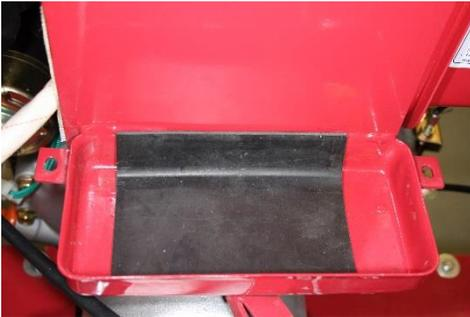
17. Place the rubber battery protector into the battery compartment.
