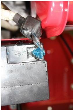
19. Screw live and neutral cables into place on battery (marked black and red on the battery). Grease the terminal and replace cover.
