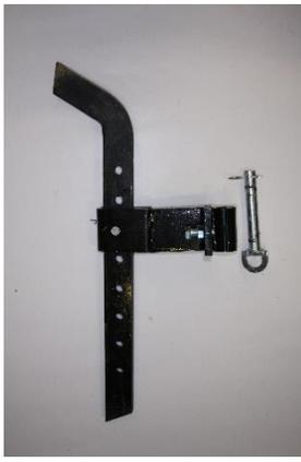
21. Place depth gauge into rear slot on machine. Adjust the pin for desired height.
