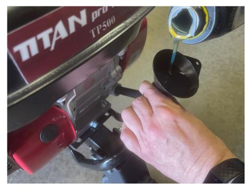
The gearbox oil should be added to the hole covered by the drain plug in the picture below. We recommend EP80w/90 GL5 gear oil; you will need approximately 1.5 litres of this. Below you can see the fill plug, whilst the first picture on the next page shows this being filled.
