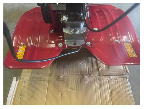
After fitting the mudguards, the next step is to install the bracket beneath these (pictured below.)
