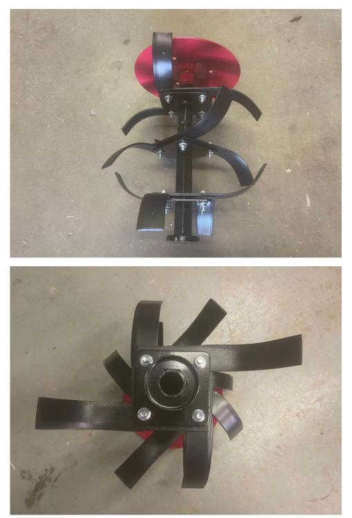
When the tines are assembled on either side of the machine, these can be fitted in place of the transport wheels we attached to the machine earlier (see page 3 of this booklet)
