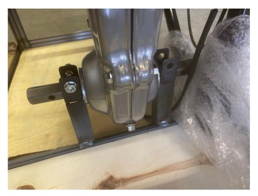
Next comes removing the chassis and engine of the machine from the cage. This will require two people to lift this out. As pictured above, the axle is bolted into two brackets to ensure the machine doesn't move in transport (one of these have been removed in the image to illustrate.) To undo these bolts, you will require a 13mm spanner, which can be found in the toolkit. After undoing these bolts, you can now lift the machine.
