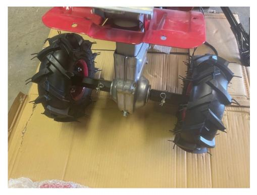
With these wheels on, you have a more solid base to assemble the rest of the unit. Next is the front wheel. The fixings (a cotter pin and a bolt, as well as washers, split pins, and castle nuts) are already in place on the wheel, so it is a case of removing these, positioning the wheel outside the bracket, and replicating how they were previously set up with the wheel in position.
