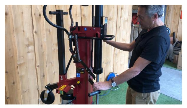
• When the ram head is down, you can then replace the cotter pin and the clevis pin in order to lock this into position.
