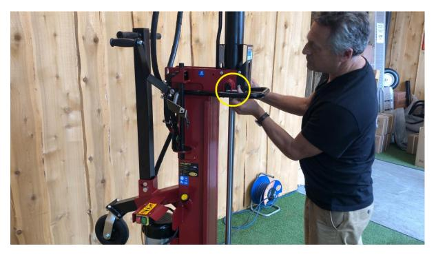
• Operate the machine per the above instructions to bring the ram head down into position.
