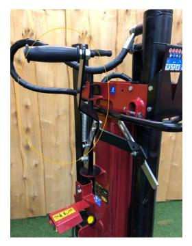
• If the motor reverses when under load, it will appear to be running, but no pressure will be developed. In this instance, please restart (switch off using the red button (circled), then switch on again (as in the first step)) your motor.
