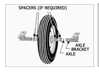
The final step is to install your new tyre onto your wheelbarrow. First, place the axle through the hub. Then, referring to step 2, check your measurements and add spacers (if required.) Finally, fasten the axle brackets.
