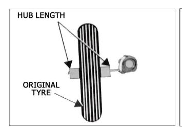
The second step is to use a tape measure to find the length of the hub. This is done by putting the tape through the axle hole to find the length, to determine how many spacers you need.
