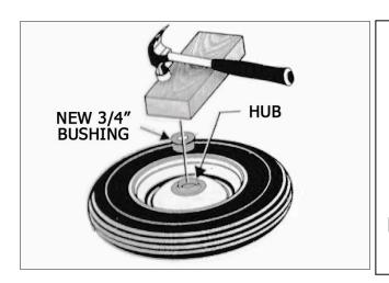
The fifth step is to insert a new bushing, should this be required.
